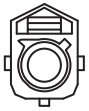
Q-016 B Camera (Front Bumper Wire Harness to Interior Floor Wire Harness Interface)
