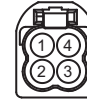
(B-198) B Interior Wire Harness to Instrument Panel Wire Harness Surround View Video Input
